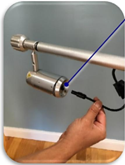
Insert Ultrasonic Unit Cable plug into back of Ultrasonic Unit
