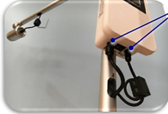
Insert Ultrasonic Unit Cable plug AND Power Cable connector into bottom of Control Unit according to printed graphic.
